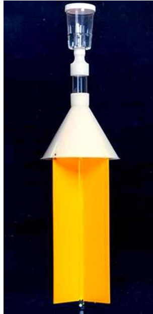
Figure 6 A cross-vane trap for monitoring brassica pod midge and its parasitoids in oilseed rape. The trap is baited with brassica-derived kairomone lures, with different compounds attracting either pests or their parasitoids. Source: AKM image.
