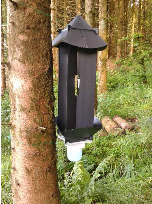
Figure 5 A cross-vane trap used for trapping bark beetles in forestry. The trap is baited with a lure, and beetles impact the vanes and fall into the collecting funnel and jar at the bottom. Source: AKM image.
