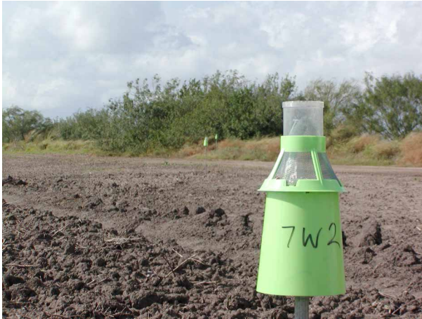
Figure 10 A boll weevil cone trap. Weevils are attracted to the colour and pheromone plume from the baited traps. Upon landing, they move upwards into the cone and are retained within the collecting jar at the top. Source: Image by Dale Spurgeon, USDA Agricultural Research Service.
