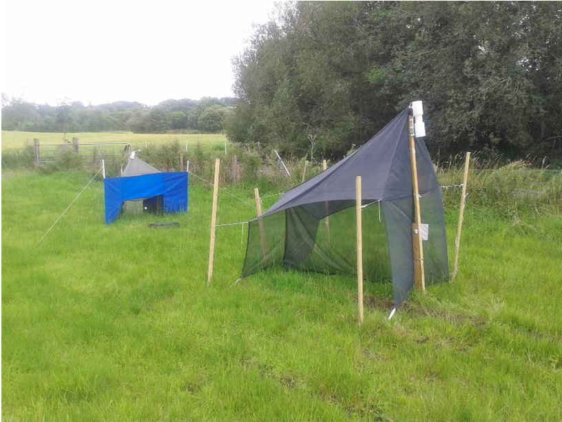
Figure 4 The Malaise flight interception trap is ideal for biodiversity sampling of flying insects, particularly Diptera and Hymenoptera. As a large, delicate and non-selective trap, its use in crop protection has mainly been for experimental studies. Source: AKM image.
